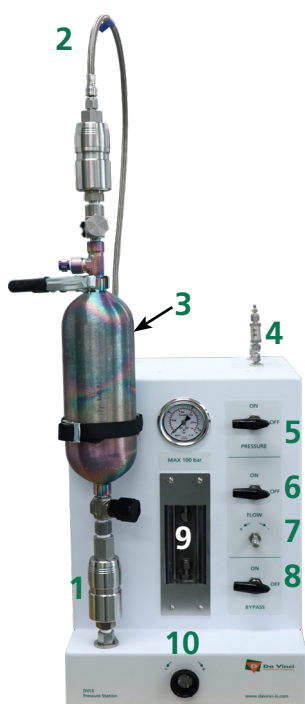
DVLS Pressure Station with Vaporizer
