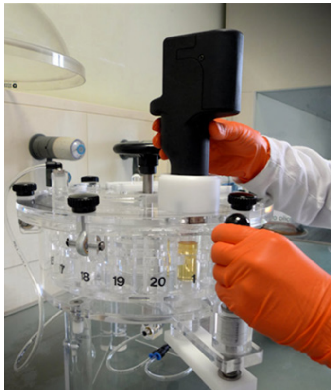
The sealing cap point with electronic crimper
